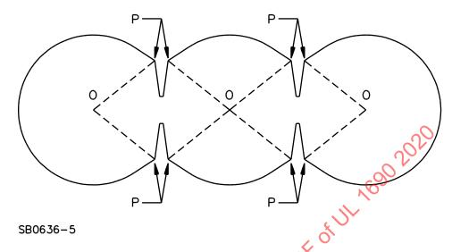
Constructions with a Cross Section Having a Definite Point P at the Outer End of Each Valley Slope OP in each case is a straight line from the center O of a conductor to P on the same segment of the cross section. Thickness measurements are not to be made on any valley slope.
