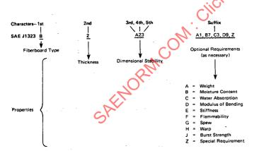
By using the breakdown in paragraph 3.5 and the tables in paragraphs 4.1 through 4.5, the example line call-out specifies a hardboard, 0.203 mm thick, with a 0.5% maximum expansion and a 0.75% maximum contraction after humidity exposure. The optional requirements include a weight of  $1 \pm 0.05$  kg/m<sup>2</sup>, a moisture content of 5–9%, water absorption of 30% maximum, and a special modulus bending requirement.
