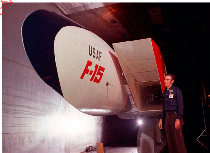
FIGURE 59 - FULL-SCALE F-15 INLET WITH MODIFIED FOREBODY
