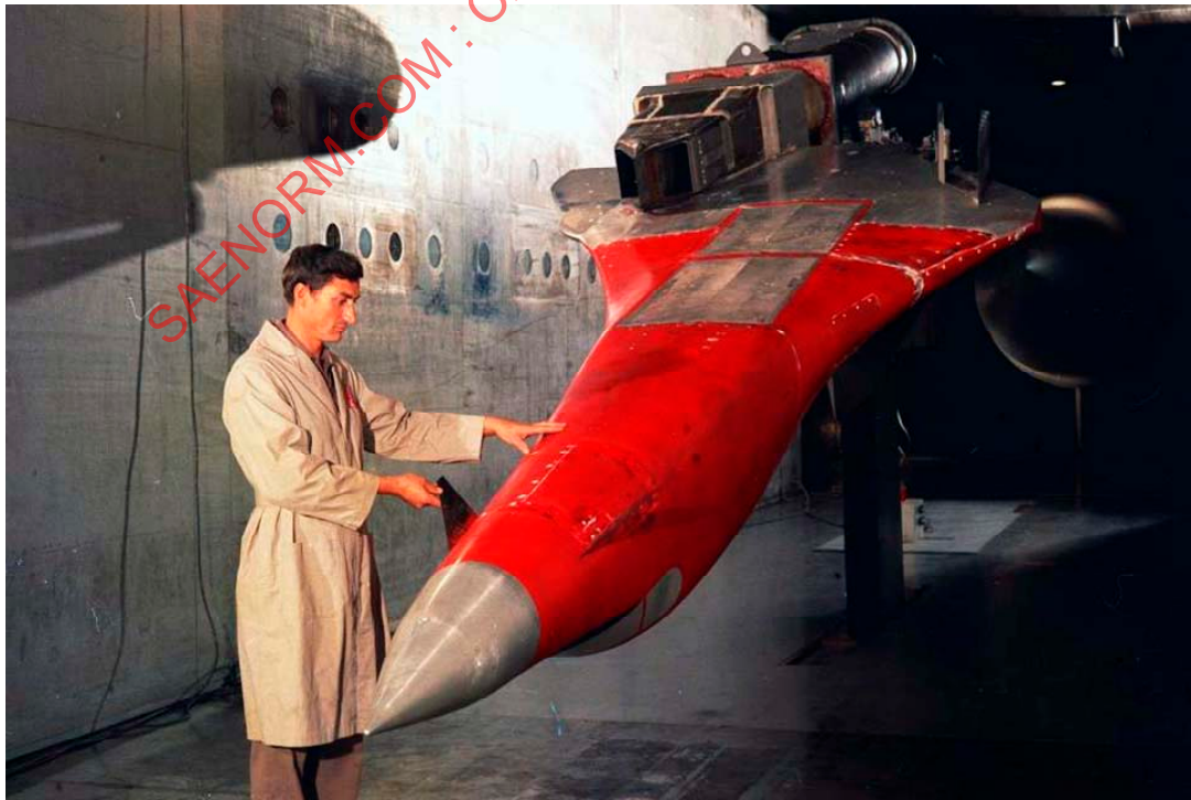
FIGURE 24 - 0.1-SCALE B-1A IN AEDC TUNNEL 16S
