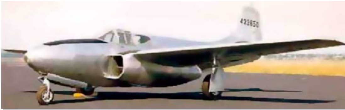
FIGURE 1 - INLET INSTALLATION OF THE BELL P-59
