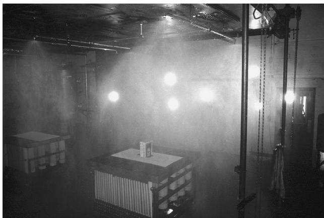
FIGURE F.3(b) Water Mist Discharge.
