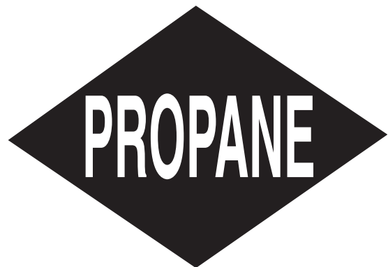
Figure 8-2.10 Example of vehicle identification marking.
