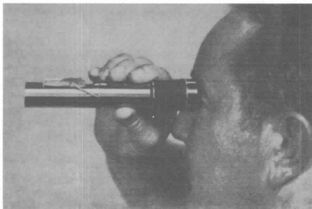
Figure 4-4.3 (b) When this type refractometer is held up to a light source, a reading is taken where the dark field intersects the numbered scale.
