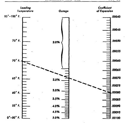
The following coefficients of expansion per degree Fahrenheit, of the principal flammable liquids shall be used in determining outages:
