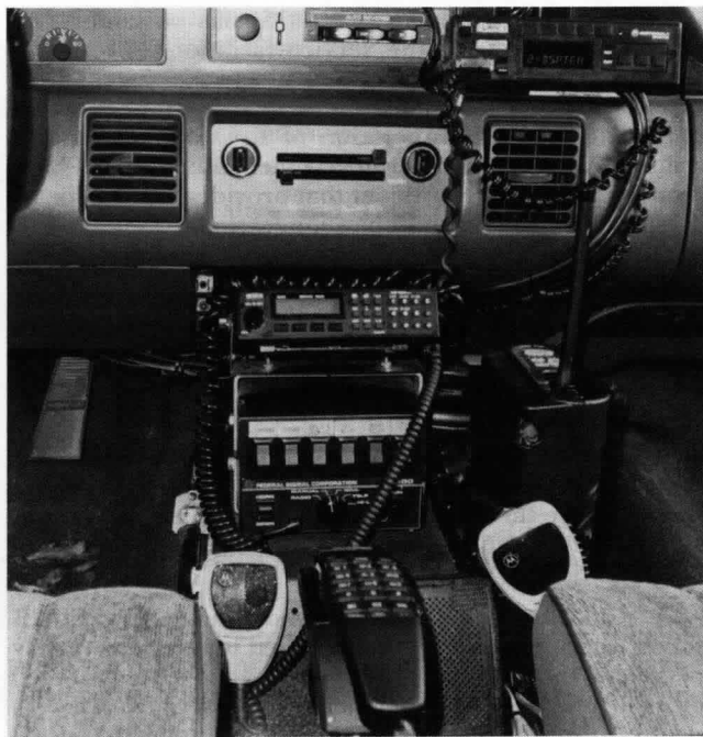
Figure 4-7(e) Multi-frequency mobile radio control head with electronic siren/public address system; and programmable scanner, portable radio with built in charger, and cellular telephone.
