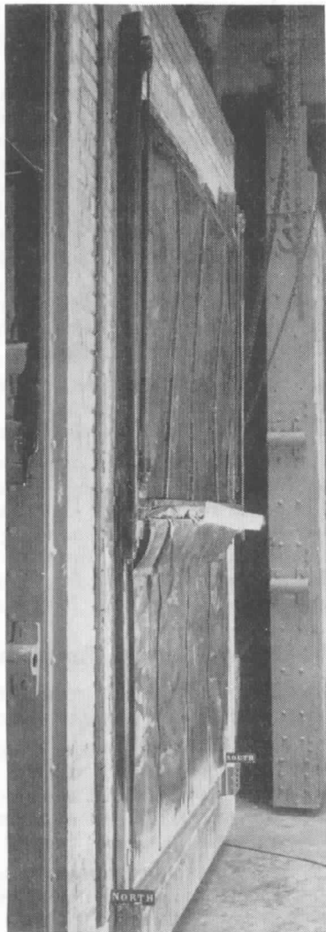
Exposed face of counterbalanced freight elevator fire door, after standard fire exposure and application of hose stream.
