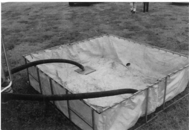
Figure C-1.13(b) Each mobile water supply should carry a portable tank that is 40 percent greater than the capacity of the mobile water supply. Note the strainer that minimizes whirlpooling and allows departments to draft to a depth of 1 in. to 2 in. (25 mm to 51 mm) in the portable tank.
