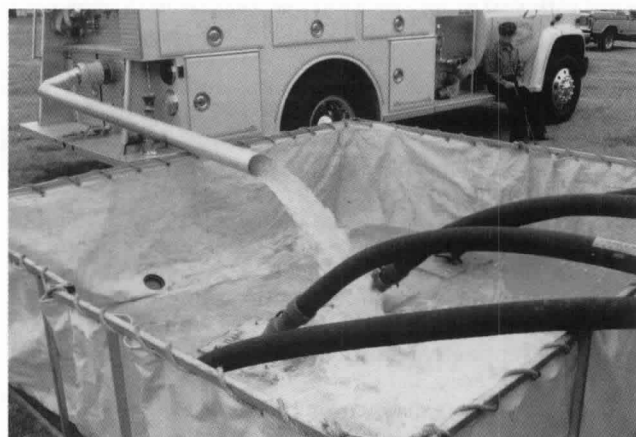
Figure C-1.14 The aluminum irrigation discharge pipe, in the shape of an “L,” allows discharge from either side or rear of the mobile water supply. Four hard suction hose lines are used to minimize any clogging of the strainers.
