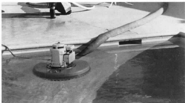
Figure E-1.2.6 Floating 500-gpm (1893 L/min) pump in swimming pool supplying the department pumper through large diameter hose.
