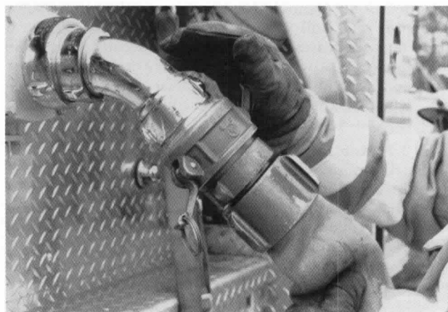
Figure C-1.11 One way to increase water-hauling capacity is to reduce the fill time of the mobile water supply. Here is one type of quick coupling that can help to reduce the fill time.
