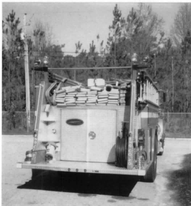
Figure D-1.6(c) Many departments have installed large diameter hose with a flat lay in the hose bed.
