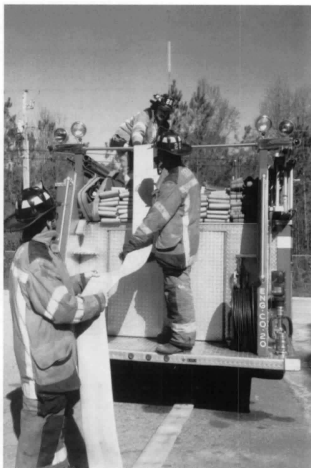
Figure D-1.6(d) Fire fighters quickly reload 5-in. (12.7 cm) hose as the apparatus straddles the hose. Note that the hose is loaded over the bar between the stanchions.
