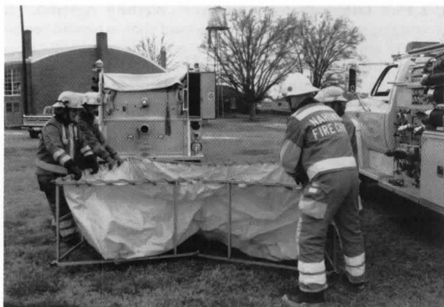
Figure C-1.13(a) Portable drop tanks should be simple to set up. Note the portable tank compartment (door open) on the mobile water supply. (Photo by Nahunta Volunteer Fire Department, NC)
