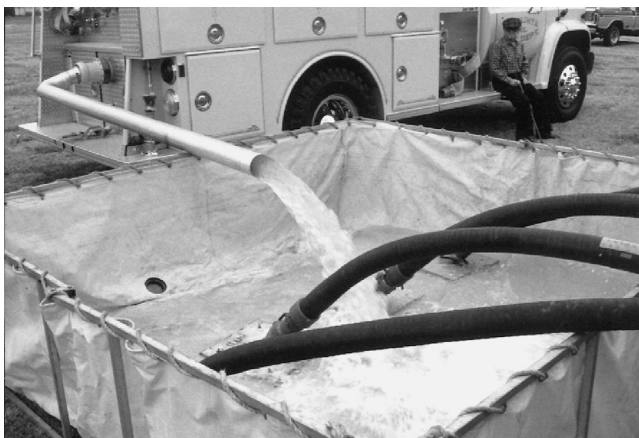
FIGURE C.14 Portable Drop Tank with “L”-Shaped Aluminum Irrigation Discharge Pipe.
