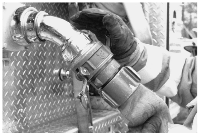
FIGURE C.10 Example of a Quick Connect Coupling That Can Help to Reduce the Fill Time.
