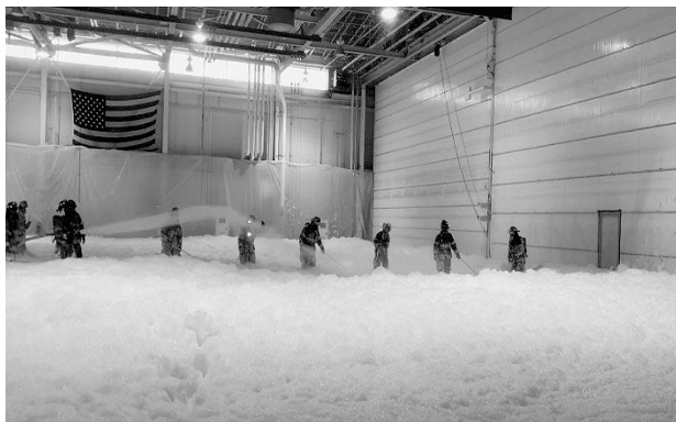
FIGURE A.7.6.3.3(c) Firefighters Sweeping 6 ft (1.8 m) Wands in a 180-Degree Motion Searching for Anything Hidden Beneath the Foam.
