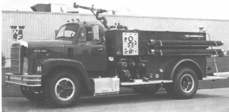
Fig. A-302(f)(1)(a). Standard foam truck-waterpump, proportioning system, airfoam concentrate tank and monitor nozzle.
