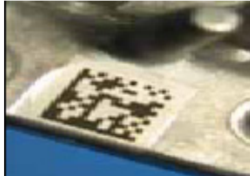
Figure A.6 — Electro-chemical etch marking on metal
