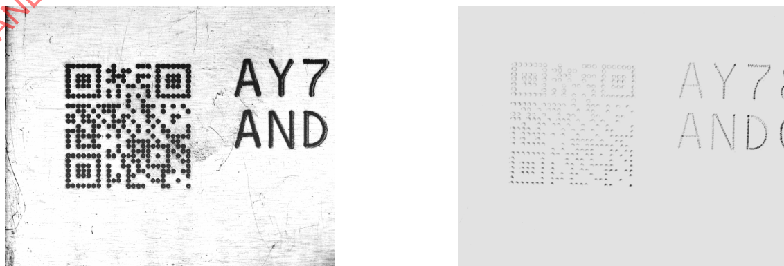
Figure A.5 — Image of dot peen marking with and without proper illumination.
