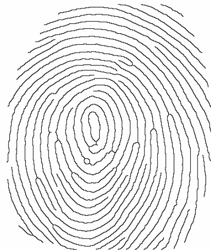
Figure E.8 — Binary image and ridge skeleton, from [14]
