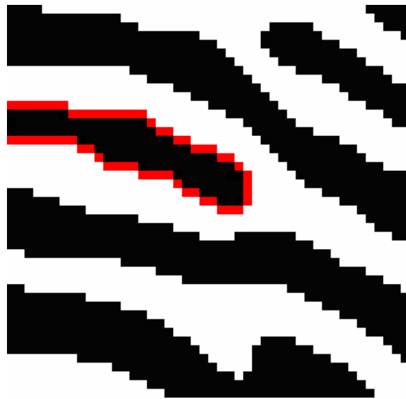
Figure E.12 — Border of a ridge skeleton endpoint
