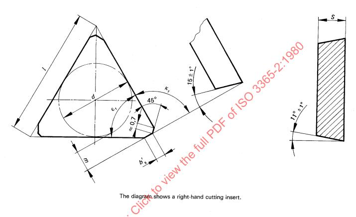
The diagram shows a right-hand cutting insert.
