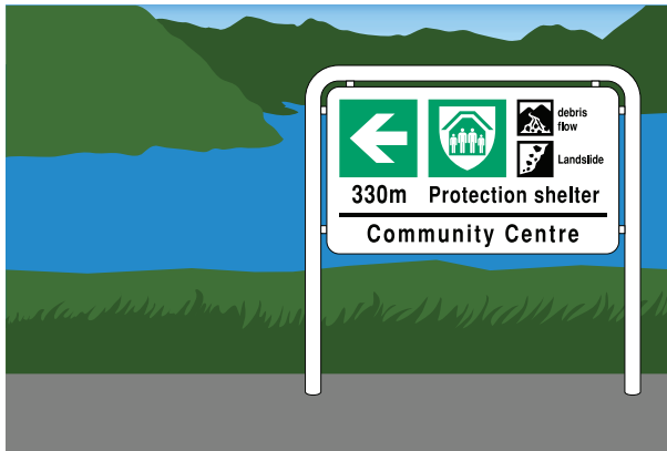
e) Self-standing debris flow and landside evacuation route sign installed on a path running along the river
