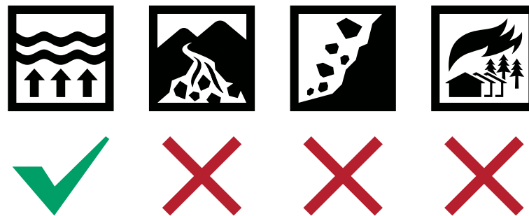
Figure 1 — Examples of markings displaying suitability for floods but unsuitability for debris flow, landslides or large-scale fires
