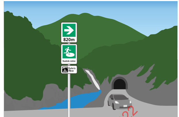
f) Debris flow evacuation route sign installed on a pole in an area surrounded by a mountain and a river
