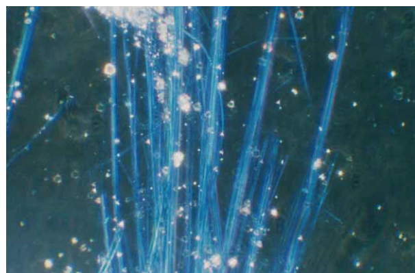
Figure D.16 — SRM 1866 crocidolite in 1,700 RI liquid — Dispersion staining — Fibre lengths normal to polarizer vibration direction
