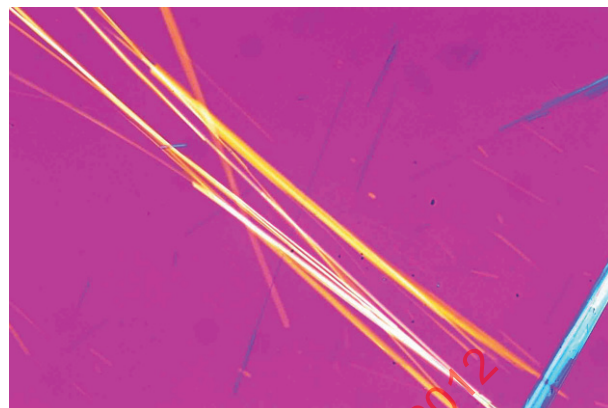
Figure D.24 — PLM micrograph of SRM 1867 tremolite in 1,625 RI liquid — Crossed polars with 530 nm retardation plate
