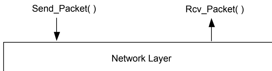
Figure 11 — Network service interface
