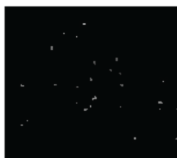
a) Cropped image from Figure B.1 with the vertical line of low-level, diffuse echoes at the flat, alumina plate's surface removed
