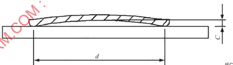
**Key** $C$  maximum concavity $d$  diameter of the flat area of the base**Figure 104 – Concavity of disc**
