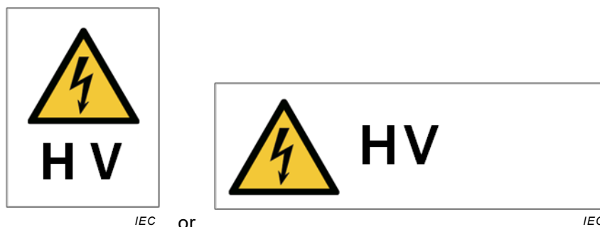
Figure 4 – Warning sign “high voltage”
